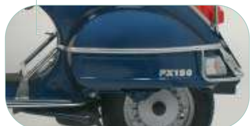
610273M Perimetrale posteriore cromato Chrome-plated rear side protection
