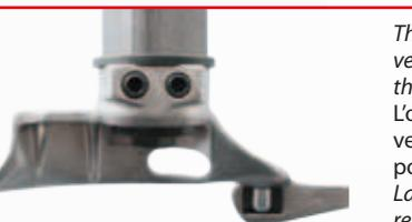
The mounting tool can be adjusted vertically and laterally displaced from the rim.
