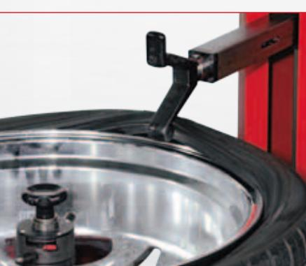
The tool in precision cast steel is completely coated with a special plastic material in order to avoid any damage in the case of contact with aluminium rims. It is located and operates on the same axis as the chuck and enables the operator to constantly control its correct position and avoid errors.
