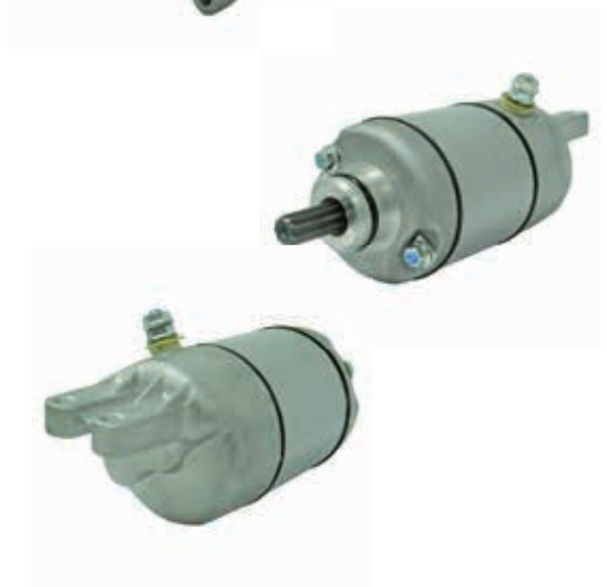
◀ cod. 19633N Mitsuba PMDD 12 Volt, CCW, 9-Tooth Pinion
