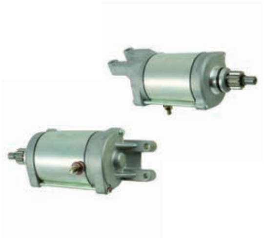
◀ cod. 18760N Mitsuba PMDD 12 Volt, CW, 12-Tooth Pinion
