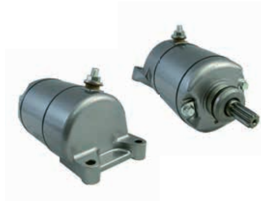
◀ cod. 18715N Mitsuba PMDD 12 Volt, 9-Tooth Spline
