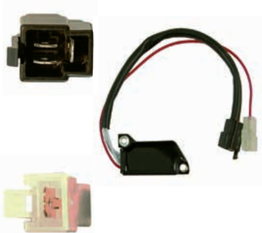
◀ cod. YM1005N Yamaha Applications 12 Volt Regulator Rectifier Assembly
