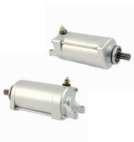
◀ cod. 18478N Denso PMDD 0.8kW/12 Volt, CCW, 9-Tooth Pinion
