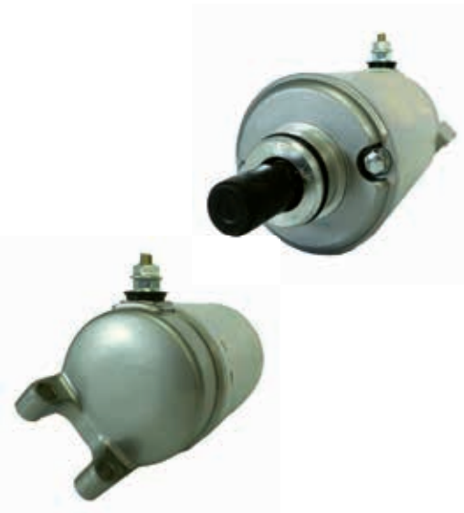
◀ cod. 19646N Denso PMDD 12 Volt, CW, 9-Tooth Pinion
