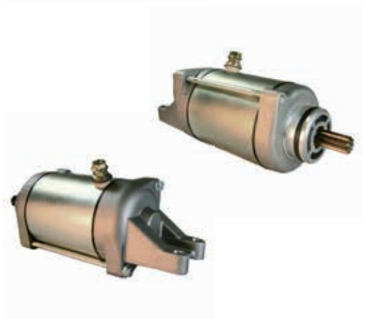
◀ cod. 18733N Mitsuba PMDD 12 Volt, CCW, 9-Tooth Spline
