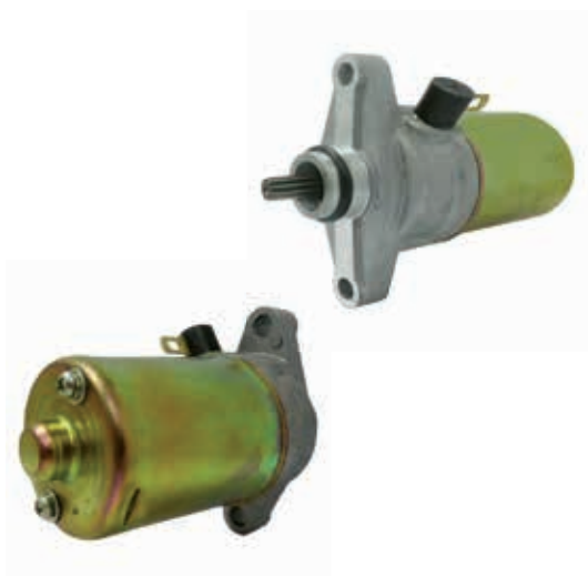
◀ cod. 19597N Chinese PMDD 12 Volt, CCW, 10-Tooth Pinion
