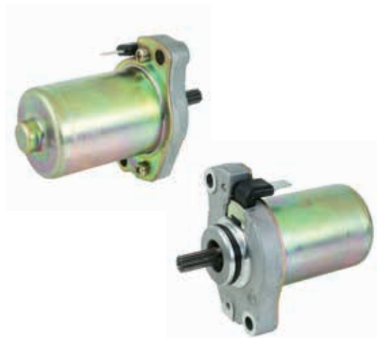
◀ cod. 18749N Mitsuba PMDD 12 Volt, CCW, 10-Spline Shaft
