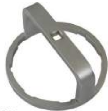
AST6052 109mm diameter / 8 Grooves 3/8" Sq. Drive CITROËN – PEUGEOT – RENAULT diesels
