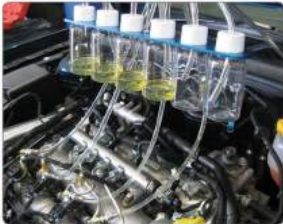
Fuel Measurement Hanging Rack Assembly.
