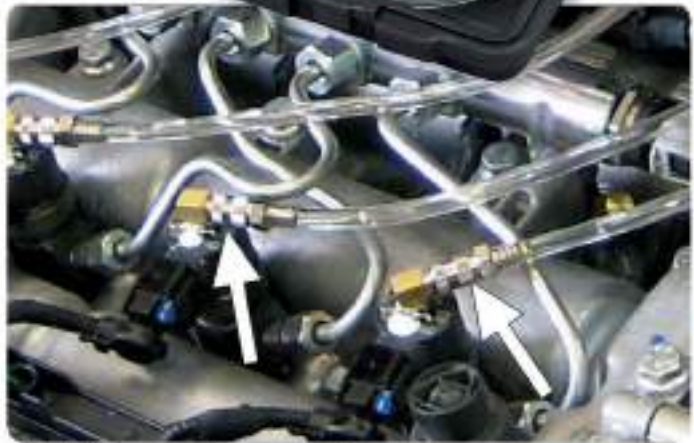
Quick Coupler Adaptor System - "No leak" connections.
