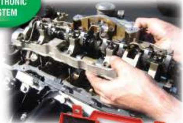
AST4800 Engine Timing, including VANOS alignment
